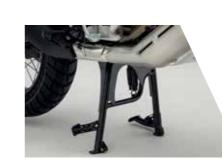
MAIN STAND 08M70-MKS-E00 The Main Stand allows secure parking on a v
