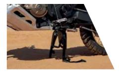
MAIN STAND OBM70-MKS-E00 The Main Stand allows secure parking on a variety of ground surfaces and assists with maintenance operations.
